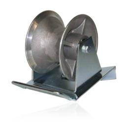
When feeding cable from a cable drum into an underground conduit system it would need to pass over the edge of the manhole into the conduit. This could cause considerable damage to the cable coating unless suitable guiding equipment is used. Also unless guiding equipment is used the winching tensions are difficult to regulate and there could be possible safety risk for the installation contractors.
